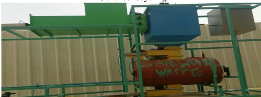
Bioreactor used to produce methane gas from organic waste to use for the purpose of heating or electricity generation
