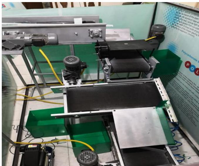
(Automatic waste segregation machine that automatically separates different kinds of wastes
