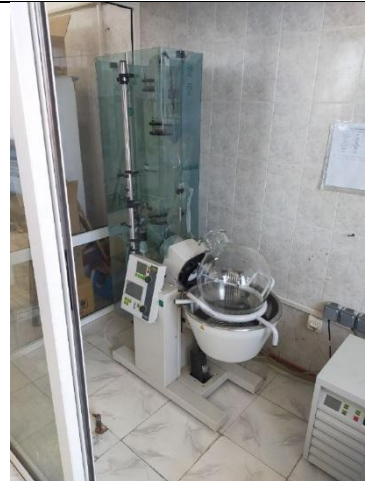
Rotary evaporator for recycling of organic solvents
