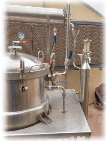
High-Performance Extraction Distillation System that recycles plant waste and convert it to natural fertelizer
