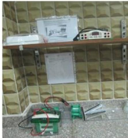
Vertical Gel Electrophoresis
