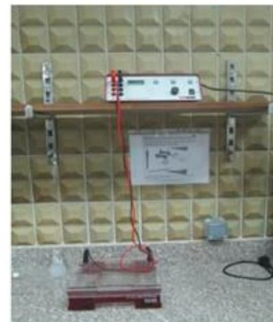
Horizontal Gel Electrophoresis System
