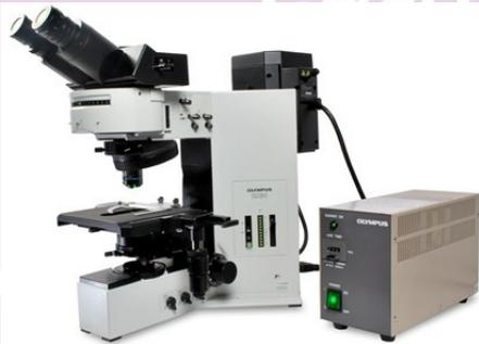
**Fluorescent microscope:** To allow visualization of fluorescent stained cells
