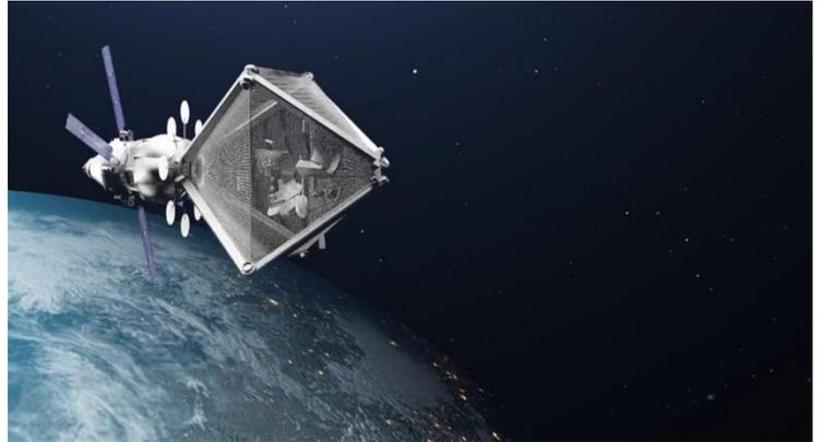
Figure 9: Robotic arms & electromagnetic mesh closed to contain the space debris
